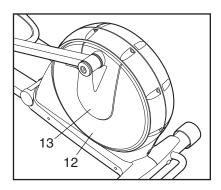
using a flat screwdriver. Next, remove the four Screws (not shown) from the center of the left Disc (12). Gently rotate the Disc Cover and the Disc away from the elliptical exerciser.
